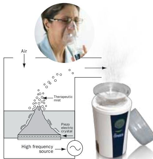
Fig 2 (b) Working of an ultrasonic nebulizer
